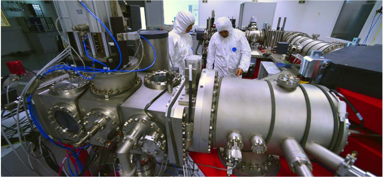
IAEA laboratory analysts use a secondary ion mass spectrometer to examine safeguards environmental samples to detect unreported activities or undeclared nuclear materials. Photo: D. Calma, IAEA.
