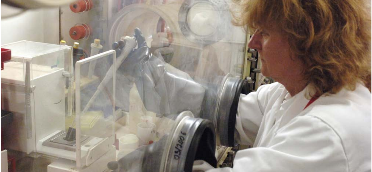
An IAEA analytical chemist measuring the plutonium content in an inspection sample. The typical accuracy for such measurements is 0.1%. Plutonium toxicity requires that such operations be carried out in glove boxes to prevent contamination. Photo: D. Calma, IAEA.
