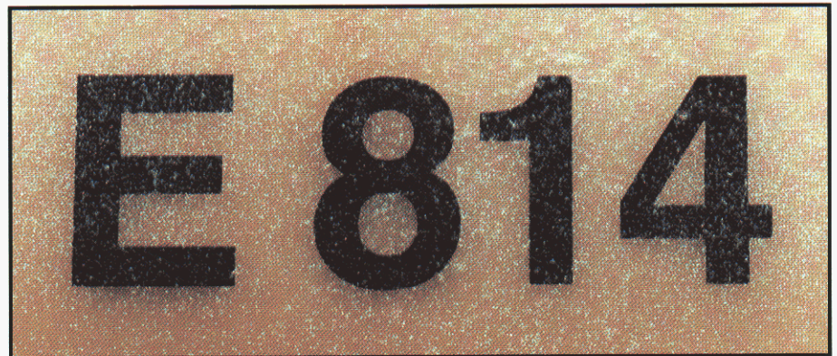
Figure 1. Reflections from light projected at various angles onto a reflective tag would uniquely identify a treaty item. The paint contains randomly oriented particles that create three-dimensional reflections, making it virtually impossible to counterfeit the tag.
