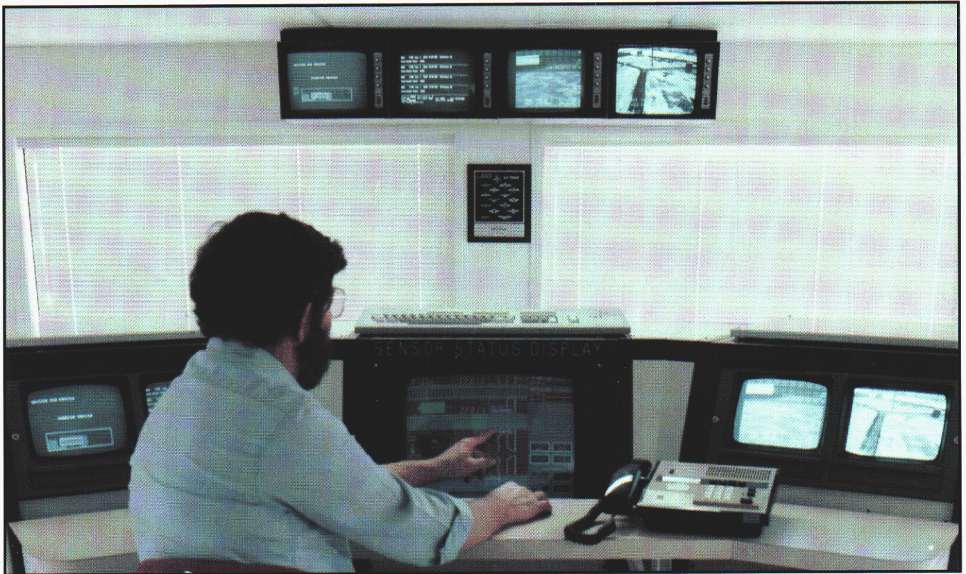
Figure 4. TV monitors and other detection equipment in both on-site portal control rooms and off-site observation centers could be used to observe the perimeter and the nature of traffic through the exit portals.
